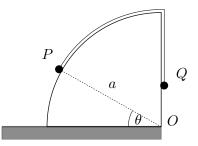
The diagram shows two particles, P and Q, connected by a light inextensible string which passes over a smooth block fixed to a horizontal table. The cross-section of the block is a quarter circle with centre O, which is at the edge of the table, and radius a. The angle between OP and the table is  $\theta$ . The masses of P and Q are m and M, respectively, where m < M.
